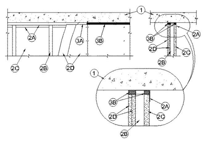
1. Floor Assembly — Min 2-1/2 in. (64 mm) thick reinforced lightweight or normal weight (100-150 pcf or 1600-2400 kg/m<sup>3</sup>) structural concrete.
